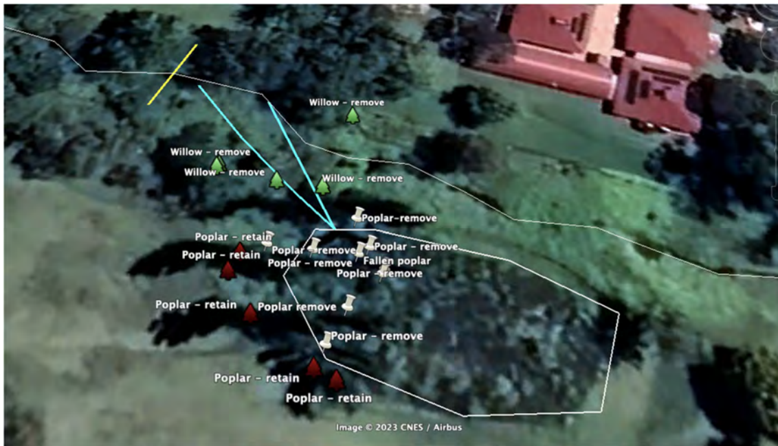
Figure 8: Tree removal in and around the dam. The white line is the approximate boundary of the dam. The blue-green lines show approximate location of new high-flow channels for flow into the dam from the creek. (Source: Google Earth.)
