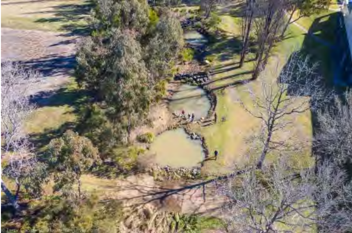
Figure 5: In Stage 2 of the Black Gully Rejuvenation, these pools were widened and protected with rock banks. Photo: Terry Cooke.
